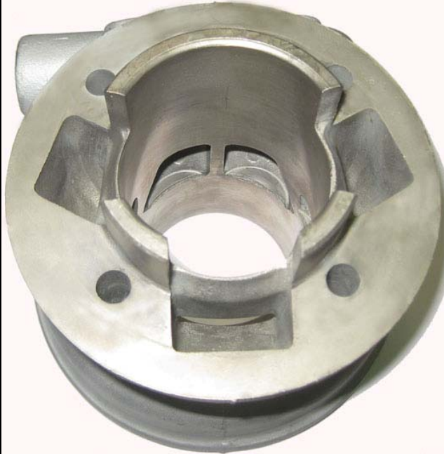
PHOTO OF CRANKCASE - GASKET FACE
